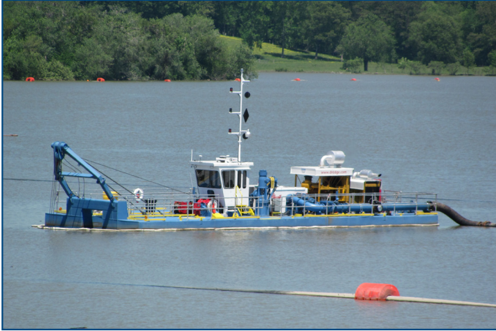
870JD 60 ft. (18 m) used for sand mining
